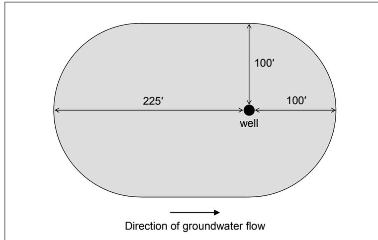
(b) Examples of possible well recharge areas for two private wells. Recharge areas represent the area of land that contributes water to a certain well. Depending on the direction of groundwater flow and well depth, recharge areas can be at different distances away from the well. Note that the distance between the recharge area and the well can vary considerably based on the predominant direction of groundwater flow. Adapted from Fig. 3 in Horsley & Witten Inc., 2000.<sup>31</sup>
